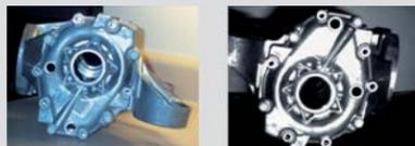
**Object: Housing assembly.** Detect presence/absence of fasteners.
