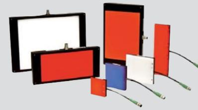
Backlights provide diffused illumination from behind the subject. They are used to outline a part's overall shape, minimize visibility of clear housings, and to view openings such as drilled holes.
